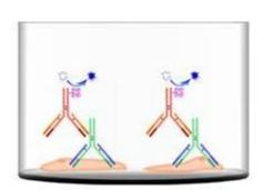
TMB substrate is converted to the blue TMB diimine via the HRP enzyme. Upon addition of acid, the reaction terminates and the wells can be read at 450 nm.
